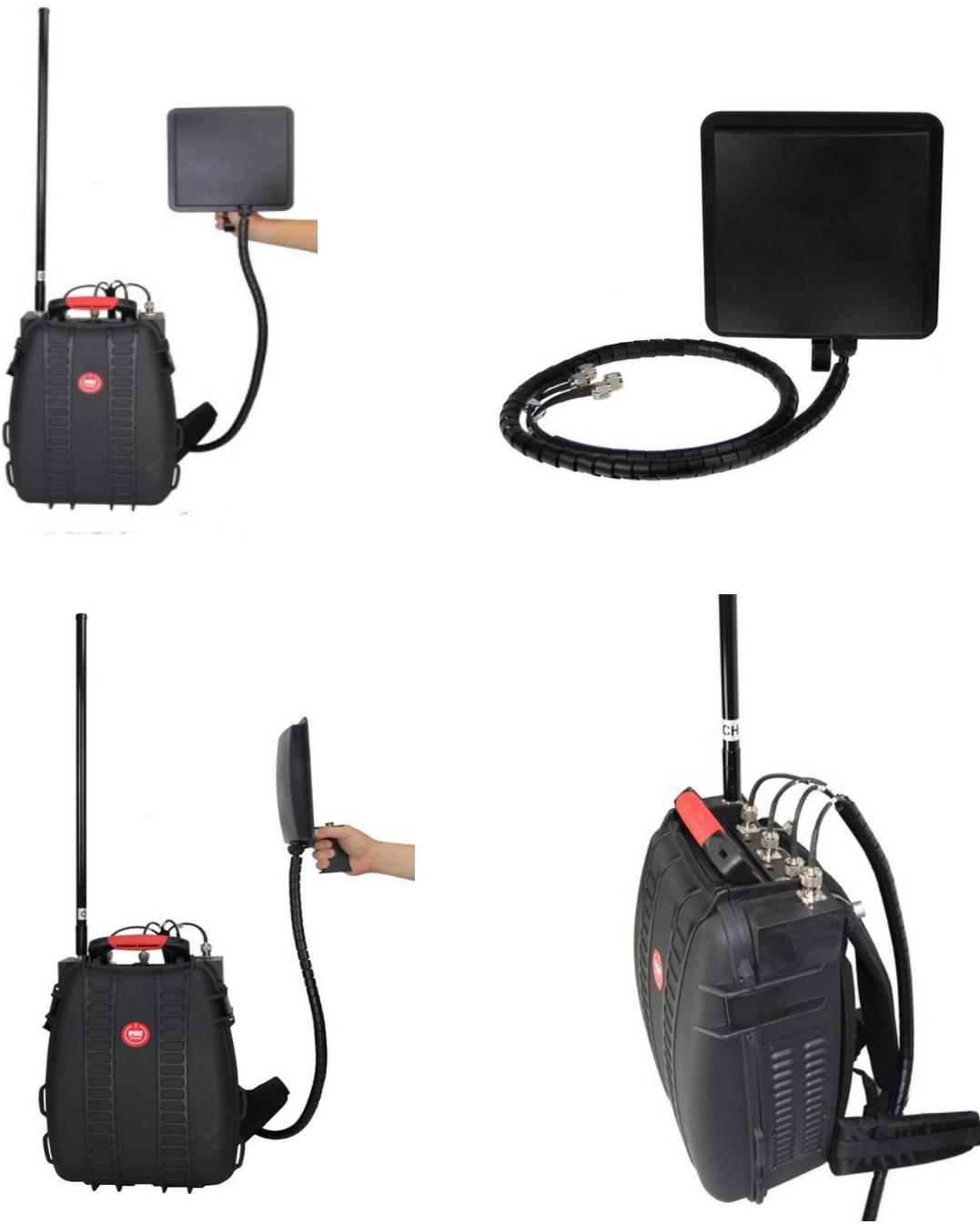
**Three 2.4GHz Bands 20W per band ( 2 bands in Directional Antenna, 1 band in Omni Antenna)**
