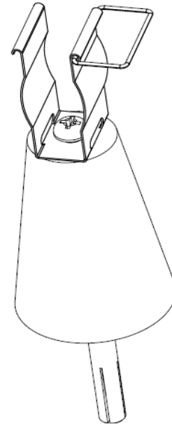
Assembly of 7/8 SS Clamp
