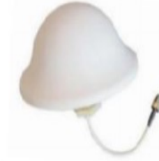
698-960/1710-2700MHz 3dBi Omni Ceiling Antenna
