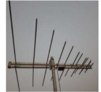
LOG PERIODIC DIPOLE ANTENNA 150-500MHz
