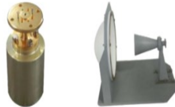
Feed Irradiation Lens Antennas
