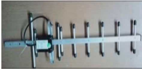
DIRECTIONAL YAGI ANTENNA - 12dBi
